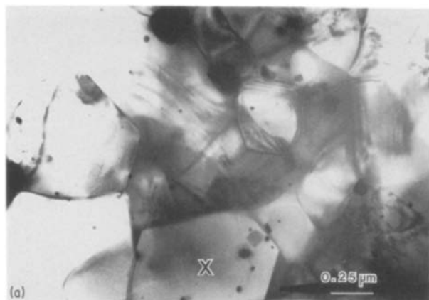
Figure 13 (a) TEM showing grain morphology on the HPSN side of the joint. The EDS spectrum (b) was taken from the grain marked X and shows the presence of a small amount of aluminium indicating that the grain is \beta' -sialon. Aluminium, 8.68 at %; silicon, 91.32 at %.
